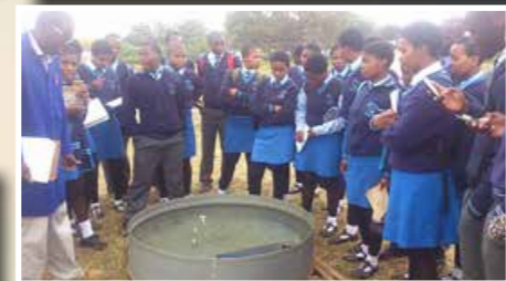
GEP technologist, Mr. M.S. Malinga taking students from Thembelihle High School through instruments kept in a Stevenson screen, and how an evaporation pan is used to estimate the rate of evaporation.
